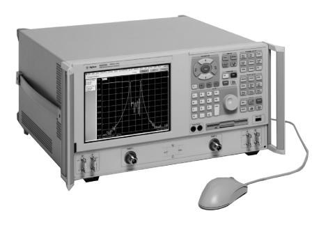
This configuration guide describes standard configurations, options, accessories, upgrade kits and compatible peripherals for the RF PNA Series of vector network analyzers. This guide should be used with the Agilent RF PNA Series Data Sheet for a complete description of these analyzers.
